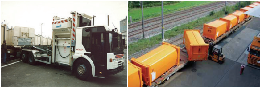
FIGURE 17 - TRANSSHIPMENT OF THE CONTAINER FROM TRUCK TO RAIL WITH ACTS SYSTEM
